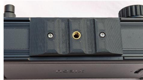
5. Attach your tripod to the 1/4-20 threaded insert in the mount. Tighten securely, but do not over tighten.
