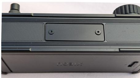
2. Remove the screws but leave the metal plate in place. **Save these screws in a safe place, you will need them should you ever decide to remove the tripod mount.**
