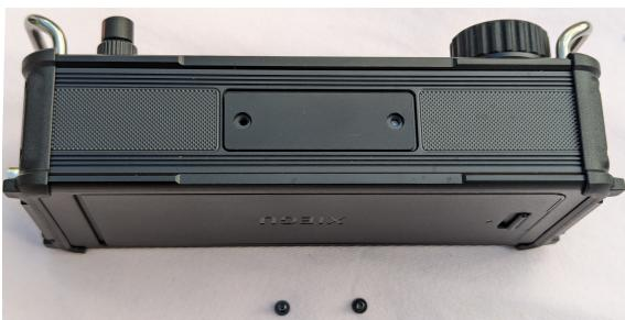
3. Line up the tripod mount with the holes in the bottom of the rig, and place the 2 M3 x 10mm screws in the holes.
