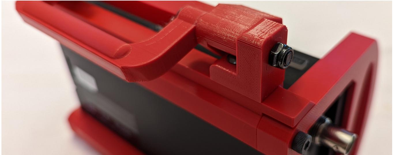
8. Now attach the screen cover to the hinge with 2 M4x8mm button head screws. Tighten these screws firmly.
