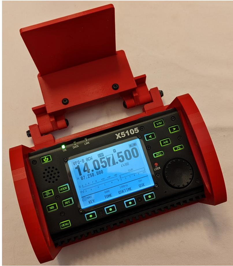
When completely assembled, you can fold the handle down and lower the screen cover to protect the screen during transport or storage of the rig.
