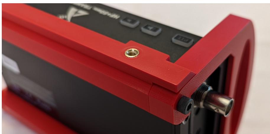
4. Attach the handle brackets to the top of the frame using the two M4 x 12mm button head screws. If you look at the L-shaped brackets closely you will notice that one leg of the L is thicker than the other. The thick leg should be vertical. Note that one side of the bracket is smoother than the other – the smooth side should face the operator. Line the brackets up with the frame and tighten the screws securely.
