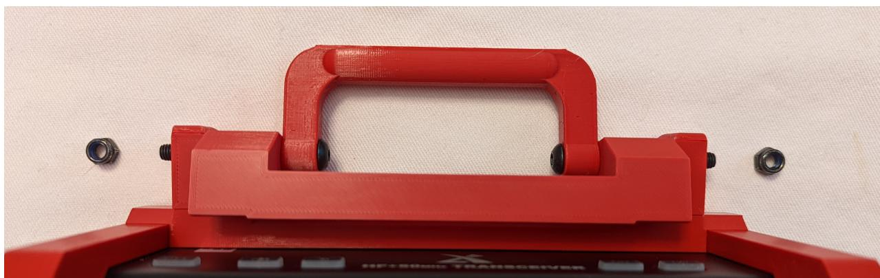
7. Now thread a nylon insert nut onto the protruding screw on each side, and tighten each with a hex key while holding the nut with an adjustable wrench or socket. The degree of tightness will affect the ease of motion of the handle and the screen cover. The nuts should be tight enough that the handle and hinge will hold the position you leave them in, but no so tight that they bind or are difficult to move. It may take a bit of experimentation to get it just right.
