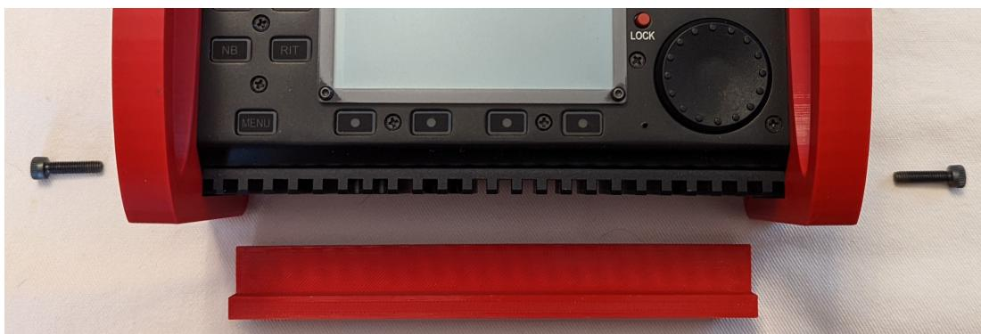
3. Attach the top rail to the side rails with two M4x16mm screws. The brass inserts in the top rail should be facing up, away from the rig.
