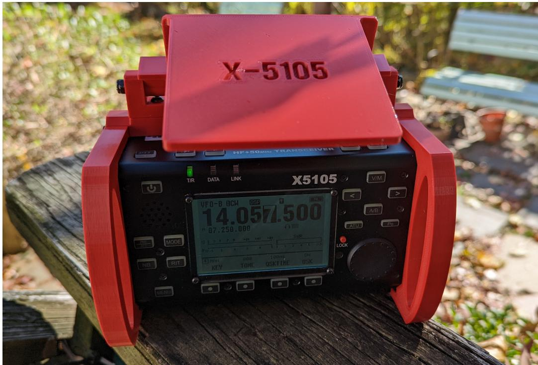
With the cover in the fully back position, you can use it as a convenient phone rest while logging or spotting on your phone. (Be sure to tighten the hinge screws sufficiently so that the cover will stay in place.)
