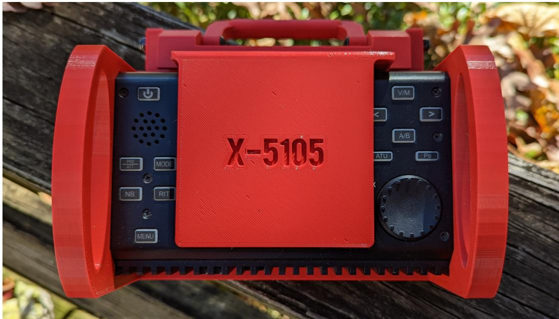
When the rig is in use, you can adjust the position of the screen cover to make an effective sun shade.
