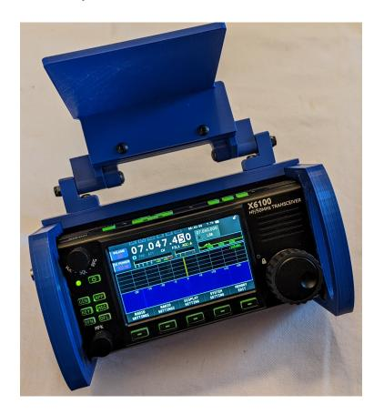
When completely assembled, you can fold the handle down and lower the screen cover to protect the screen during transport or storage of the rig.
