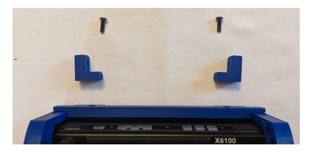
5. Assemble the hinge and handle by inserting the M5 x 45mm button head screws from the handle into the hinge.
