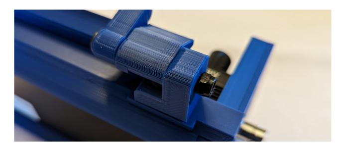
8. Now attach the screen cover to the hinge with 2 M4x8mm button head screws. Tighten these screws firmly.
