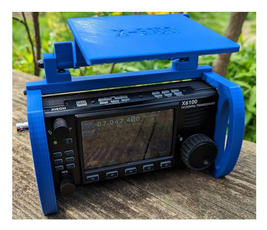
With the cover in the fully back position, you can use it as a convenient phone rest while logging or spotting on your phone. (Be sure to tighten the hinge screws sufficiently so that the cover will stay in place.)
