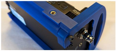
4. Attach the handle brackets to the top of the frame using the two M4 x 12mm button head screws. If you look at the L-shaped brackets closely you will notice that one leg of the L is thicker than the other. The thick leg should be vertical. Note that one side of the bracket is smoother than the other – the smooth side should face the operator. Line the brackets up with the frame and tighten the screws securely.
