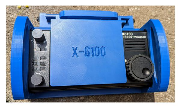
When the rig is in use, you can adjust the position of the screen cover to make an effective sun shade.
