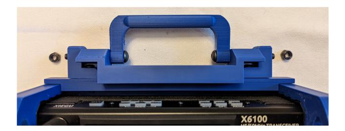
7. Now thread a nylon insert nut onto the protruding screw on each side, and tighten each with a hex key while holding the nut with an adjustable wrench or socket. The degree of tightness will affect the ease of motion of the handle and the screen cover. The nuts should be tight enough that the handle and hinge will hold the position you leave them in, but no so tight that they bind or are difficult to move. It may take a bit of experimentation to get it just right.
