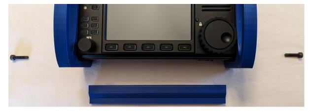
3. Attach the top rail to the side rails with two M4x16mm screws. The brass inserts in the top rail should be facing up, away from the rig.
