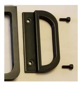
2. Attach the handle brackets to the top of the frame using the two M4 x 12mm button head screws. If you look at the L-shaped brackets closely you will notice that one leg of the L is thicker than the other. The thick leg should be vertical. Note that one side of the bracket is smoother than the other – the smooth side should face the operator. Line the brackets up with the frame and tighten the screws securely.
