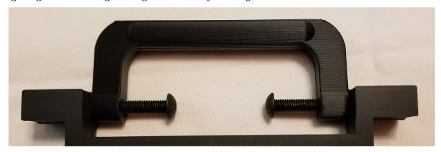
4. Now place the handle and cover assembly inside the brackets you mounted on the frame in step 2. Line up the holes in the bracket with the M5 screws, and push the screws all the way through so they protrude through the brackets on both sides. This is easiest to do if you hold the cover flat against the front of the rig.
