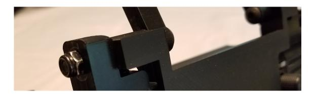
6. Attach the bottom bracket to the radio using 4 M4 x 16mm stainless button head screws. The front of the bracket is jogged a bit to accommodate the bezel of the radio. When installed correctly you should see the bright brass inserts facing you. Tighten these screws firmly, but do not use excessive force.
