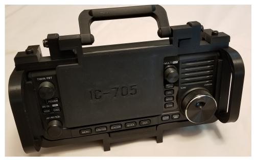
When the rig is in use, you can adjust the position of the screen cover to make an effective sun shade.
