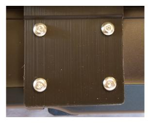
7. Start attaching the frame to the bottom bracket using 2 M4 x 10mm socket head screws, but **do not tighten these screws at this time.** They should only be screwed in far enough to remain in the holes. We will tighten them in a later step.
