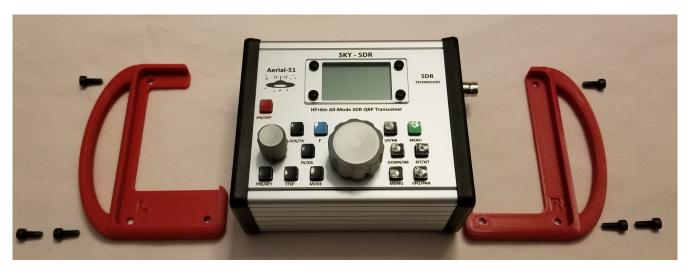
Identify the side rails – they are marked "L" and "R" referring to the left and right sides of the rig as you look at it from above.
